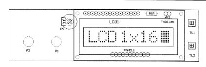
Fig 10: Component layout of the display PCB.
