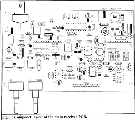
16 pins to the front panel. Secure the potentiometers P1 and P2 by fitting the shaft nuts.
